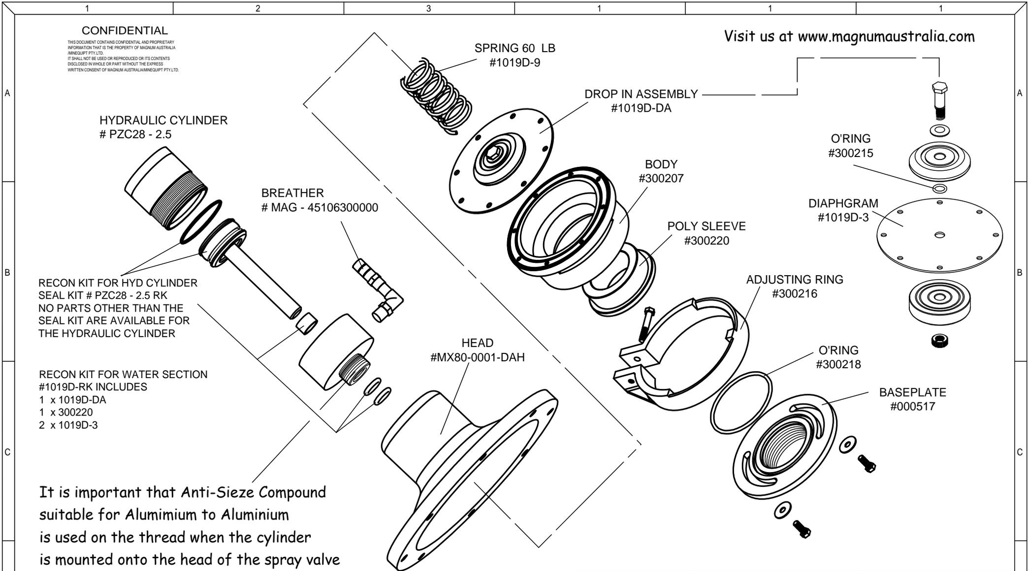
It is important that Anti-Sieze Compound suitable for Alumimium to Aluminium is used on the thread when the cylinder is mounted onto the head of the spray valve
